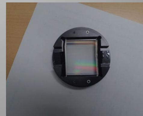
Grating: 300 Grooves / mm, VIS, Edmund opt.
